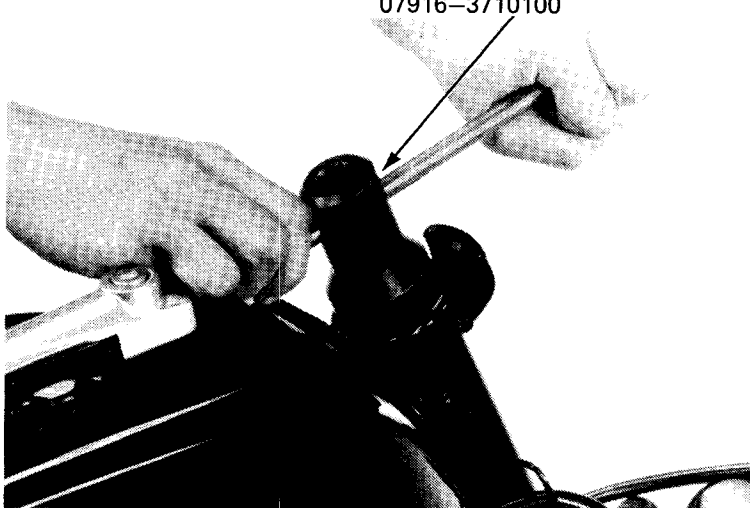
STEERING STEM SOCKET 07916-3710100
